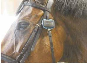
SeeHorse wearable device transmits information such as temperature, pulse and respiratory rate to a cell phone.
