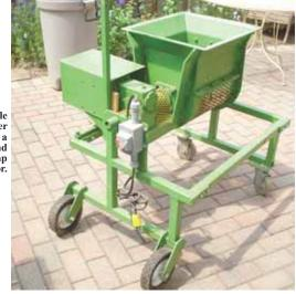
Home-built portable topsoil screener mounts on a 4-wheeled frame and is operated by a 1 hp electric motor.
