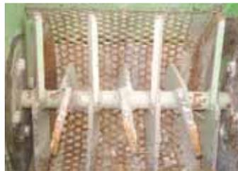
Dirt is broken up and forced through screen at bottom of drum by a revolving shaft with 1/2-in. thick steel blades welded onto it.
