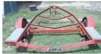
John Drew built a 6 by 14-ft., 2-wheeled flatbed trailer out of a used boat trailer. He spaced four 3-in. angle irons across the frame and welded them in place.
