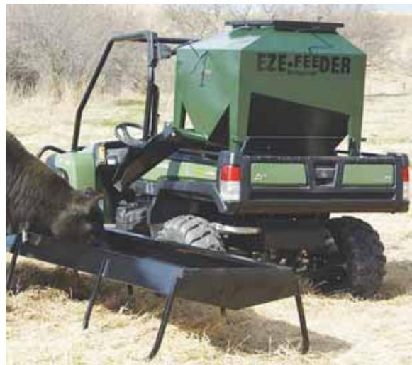
**Utility vehicle-mounted grain feeder holds the equivalent of 29 5-gal. pails of feed. Unit's 12-volt electric auger can be remotely-controlled from the cab.**
