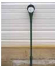
A wood rod runs from the funnel down to a float mechanism at the bottom. The rod drops with the water level.
