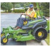
Tweel airless tire uses a solid inner hub surrounded by polyurethane spokes assembled in wedge patterns.
