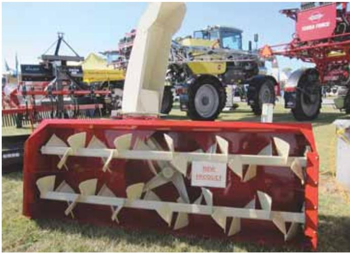
Farm King's new "Propeller series" snowblower comes with aggressive propeller blades mounted on a paddle-style auger to cut through hard-packed snow.
