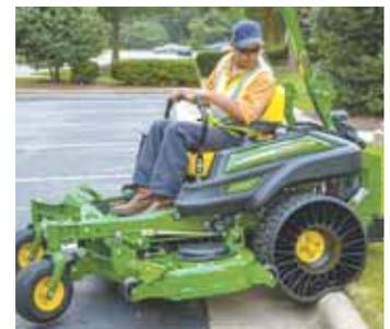
Tweel airless tire uses a solid inner hub surrounded by polyurethane spokes assembled in wedge patterns.
