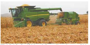
Hillco's Single Pass Round Bale System for Deere combines produces corn stalk bales that contain husks, cobs, leaves and any excess kernels exiting rear of combine.
