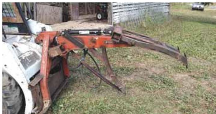
Kerry Kligora used the 3-pt. hitch frame from a scrapped-out Deutz rotary rake to build his heavy-duty log grapple. It quick-taches to his Bobcat skid loader.
