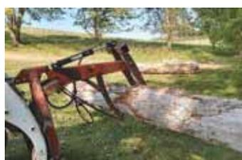
Grapple uses a pair of 3-ft. long curved, movable jaws spaced 12 in. apart, and 2 fixed shanks.
