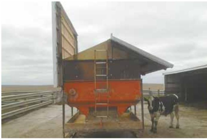
Mark Burlage converted a gravity box into this high-capacity cattle feeder. One of its roof panels tip open easily for filling with help from cinder block counterweights.
