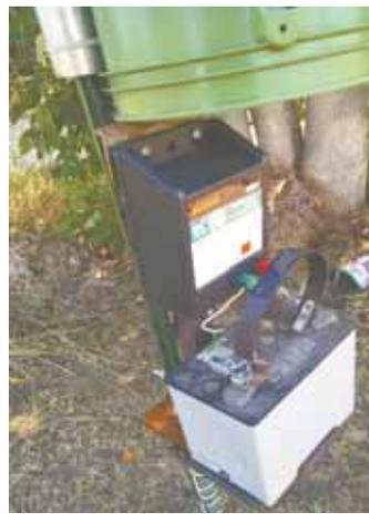
Craig Spierling uses an upside down 5-gal. pail to provide weather protection for an electric fencer. Bucket slides up and down a metal T-post. Photo at left shows pail lifted.
