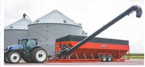
Harvest Link is a 3,000-bu., 56-ft. long holding tank on wheels that can be towed on a 3-pt. hitch. Auger has a 36-ft. reach and both fore and aft motion, allowing it to fill the length of a semi trailer.
