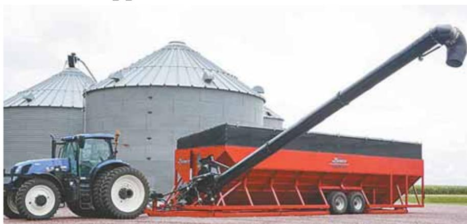
Harvest Link is a 3,000-bu., 56-ft. long holding tank on wheels that can be towed on a 3-pt. hitch. Auger has a 36-ft. reach and both fore and aft motion, allowing it to fill the length of a semi trailer.
