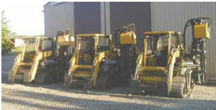
Instead of drilling holes for posts or driving them into the ground, the machine uses vibration to set 4 to 5-in. posts in less than 10 seconds.
