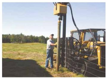
One Pass Fencemaker is a tracked vehicle with a post carrier in front and an automated fencing system attached to its side.
