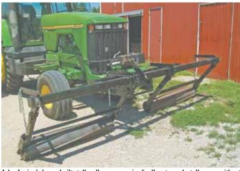
John Janing's home-built stalk roller uses a pair of rollers to push stalks over without snapping them off.
