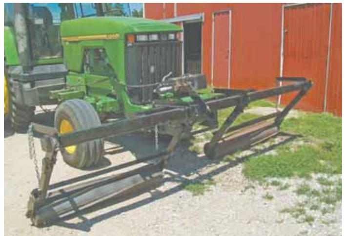
**John Janing's home-built stalk roller uses a pair of rollers to push stalks over without snapping them off.**
