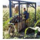
hydraulic reservoir for the pump. The 8-ft. high rig will clear 10-ft. high corn stalks with no problem.
