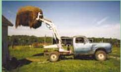
Russell Morrison of Weatherby, Mo., mounted a frontend loader on the back of his Dodge pickup. A pair of electric-over-hydraulic pumps mounted behind the cab provides lifting power. "It lets me get to distant fields at highway speeds and loads bales faster in the field," says Morrison. Best of all? He gets to ride in comfort. See page 3.
