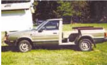
the cab behind the front seat and cut a hole in the rear of the cab with a chop saw so I could install a Plexiglas window. A shop-built 4 by 6-ft. wooden box slips in the back of the vehicle between the wheel wells. It's ideal for holding fence-fixing tools, rocks, sticks, etc. Cost only about \$100, including new battery, water pump and oil seal.
