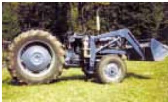
tor loader that I bought used for \$400. The hardest part was making hanger brackets to fit the front and rear of the engine. A Vickers hydraulic pump off an old shop-built hydraulic press drives off the engine crankshaft. A surplus stainless steel fire extinguisher, with 1 1/2-gal. capacity and pipe fitting brazed in the bottom, mounts upright on the rear stanchion of the loader to serve as a reservoir.
