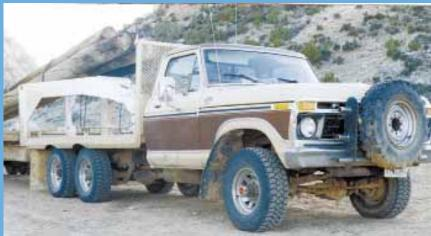
Dan Hampton of Ten Sleep, Wyo., converted a 1977 Ford F-250 3/4-ton 4-WD pickup into a 6-WD model equipped with walking beam rear axles and a 12-ft. steel flatbed. "It's a great all-around ranch truck for hauling hay, machinery, and livestock. I've hauled loads weighing up to 33,940 lbs. gross," he says.
