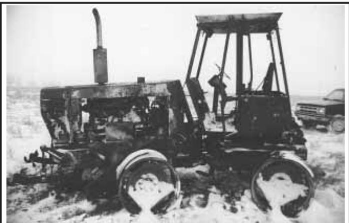
Insurance investigators believe the fire that destroyed this Ford-New Holland bi-directional tractor started in the wiring.
