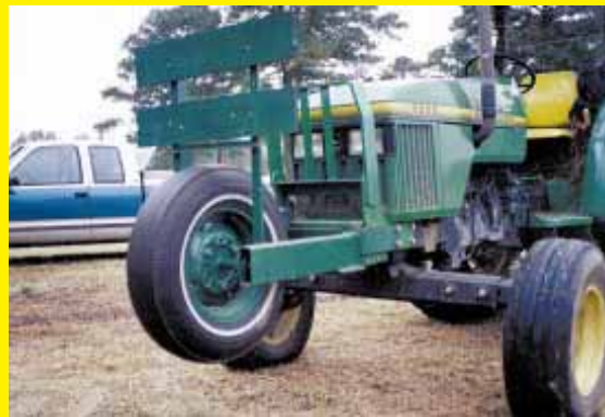
A pair of Florida farmers have come up with a way to mount a powered wheel on front of tractors to unroll round bales on the ground. The up-front wheel is powered by a hydraulic motor. "It rolls out hay like a red carpet," they say. See page 2.
