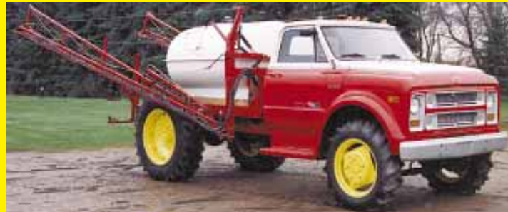
Bill Wahouske's truck-mounted sprayer is equipped with tractor tires for improved flotation and traction. "It'll walk right through the biggest mud holes and never get stuck," he says. See page 2.
