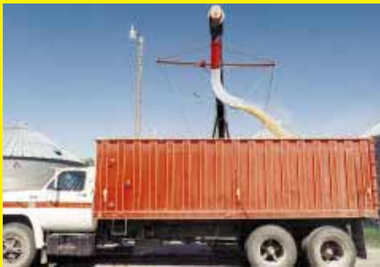
"No matter how big the truck or how it's positioned beneath my auger, I can always fill it completely full without having to move the truck," says Tim Lindhorst about his "side swing" auger unloading spout. It's controlled by a 12-volt electric winch. See page 2.
