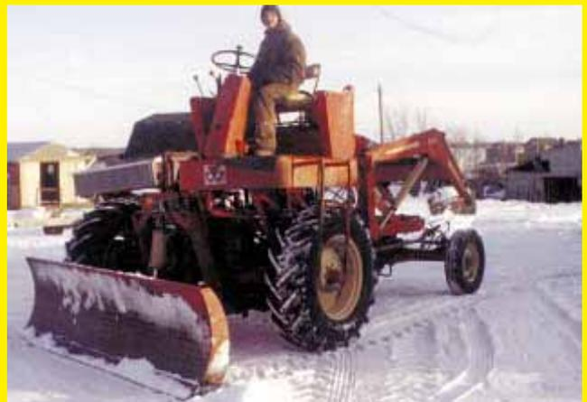
Here's a self-propelled bale hauler I built out of an old combine, a front end loader and various other components I had around the farm. It's a lot handier for hauling 5 by 6-ft. round bales weighing up to 1,000 lbs. than the tractor and dilapidated front end loader we used before.
