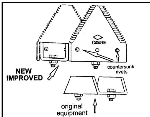
Sickle sections are riveted to original equipment so they can be reversed as they wear or replaced if they're broken.
