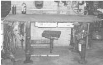
larger 4 1/2-in. dia. piece of pipe that slips up and down one of the legs so it can be positioned wherever needed by simply tightening set screws. It's useful because I can raise it up above the table or align it with the top of the table.
