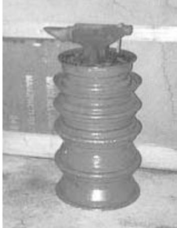
16-in. dia. wheel rims on top of each other, with one 14-in. wheel on top. All are welded together. Then I bolted an anvil to the top. Makes a solid, heavy stand that will take all the pounding you can dish out yet you can also roll it around the shop, if necessary."
