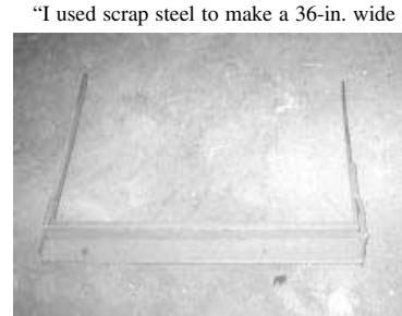
"I used scrap steel to make a 36-in. wide metal bender that lets me bend sheets of metal at a 90 degree angle. It's equipped with a hinged handle on each side. I place the bender in a vise with the handles straight up in the air. Then I slip the metal sheet in under a bar and use a pair of vise grips to keep the sheet in place. To make the bend I simply pull both handles back toward me. I copied it off a photo of a commercial unit. It makes a nice clean 90 bend."
