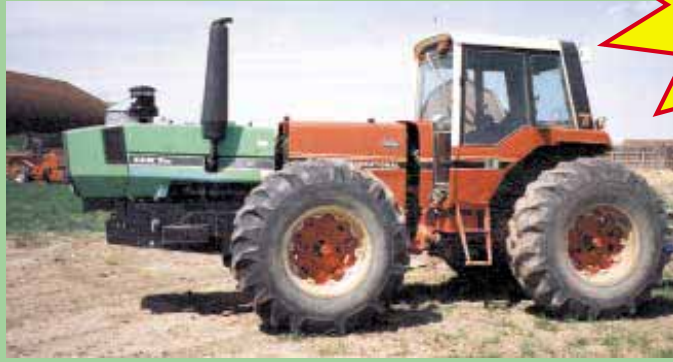
When the engine went out on his 3788 Case-IH tractor, Ken Adams transplanted the front end off a Deutz diesel right onto the frame. See story on page 2.
