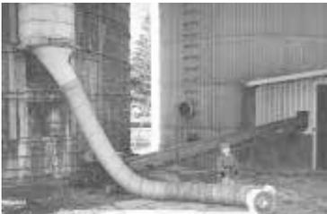
**Home-Built Silo Gas Exhaust System** – "We wanted a way to suck gases out of silos before going in," says an Ontario farmer who designed and built a system that pulls poisonous gases out of silos through the chute. It consists of a commercial 3/4 hp, 12-in. dia., high speed aeration fan from a feed bin and 25 ft. of industrial ductwork. "The first time I flipped the switch, a big cloud of orange chlorine gas was drawn out so I knew it worked."
