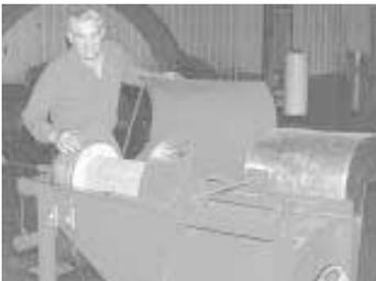
**Do-It-Yourself Air Filter Cleaner** – After he got frustrated trying to clean air filters on his equipment, an Alberta farmer decided to build his own air filter cleaner that uses a compressor to blow dust out and a large squirrel cage fan to vacuum it away. The filter is placed inside a metal housing. A 2-in. dia. pipe with holes in it blasts air through the filter from inside and a fan sucks the dust away.
