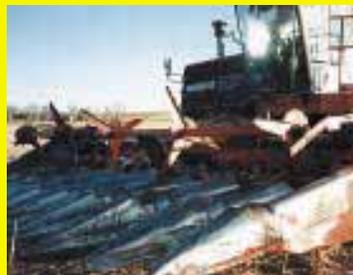
I used the center tube, mounting arms, and several of the spokes from a batt reel off an old 20-ft. wheat table. The tube was just the right length for my combine's 8-row corn head. I added several 16-in. wide, 24-in. long paddles which I made from continuous belting off a conveyor. I positioned the paddles and spokes over the row snouts, instead of the rows, so as not to impede the harvest of standing corn. The reel is driven by a hydraulic motor from the wheat table and is manu-
