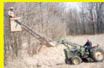
own loader-mounted cherry picker. I use it on my Deere 2020 tractor. It consists of a treated plywood box that pivots at the end of a pair of 12-ft. long steel arms that bolt to steel brackets that wrap around the box. A pair of cross pieces connect the arms together. To keep the arms from bending I attach a pair of chains to the top cross piece and down to hooks welded on back of the bucket.
