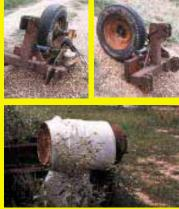
securely in place on one side by an auto hub on an arm. The tire is friction-driven by a 2-in. dia. pipe that turns against it. The pipe mounts on pillow block bearings and is driven by a small hydraulic motor that connects to tractor hydraulics.
