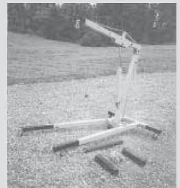
**They fabricated four new parts to convert the rolling engine hoist into a 3-pt. mounted crane.**
