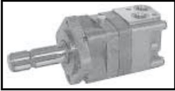
have a pto. It can also provide power in remote applications. You can use it on a tractor that already has a pto to provide a second pto. If your tractor doesn't already have a pto you can use tractor hydraulics to drive the motor. Even if the tractor does have a pto, you can mount the hydraulic-operated motor directly on an implement and not have to use the pto shaft.
