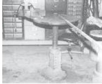
I bolted a vise onto one side of the table and use it to 'lock' an object in place, such as a length of angle iron, so that I can cut it. Works great when used together with my TV dolly. The round plate spins freely and will automatically line the vise up with the dolly.
