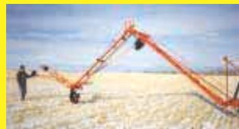
two wheels on each side of the boom, and at each end there's a small wheel to keep the boom ends from gouging into
