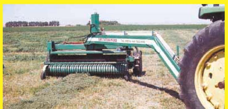
Last year FARM SHOW published an article on our add-on conditioning rollers designed to crush hay stems to cut drying time in half (Vol. 23, No. 2). The rollers are designed to replace rollers on most models of swathers and mower-conditioners. However, they don't fit all models. To meet the need we've just introduced our own 8-ft. pull-type conditioner as a stand-alone unit. The PT 8000 is designed as a followup conditioning system for use behind your swather or mower.
