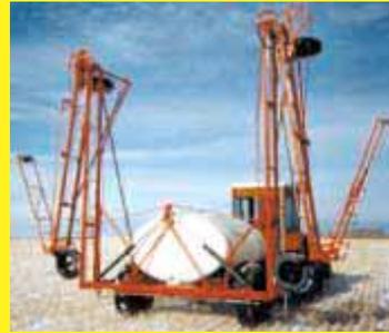
using parts from a wide variety of sources. The wings are off a Crustbuster grain drill and the main frame is off an old Deere row crop cultivator. The axle and tires are off a Cockshutt self-propelled combine and the booms are off an old sprayer that I already had. The 500-gal. tank and the sprayer pump and pto are new. There's no fancy computerized controls on it - to operate it I simply reach through the tractor's back window.
