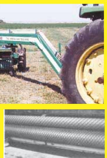
All models make use of a unique air bag pressure system that holds the rubber-coated steel rollers tightly together. As the crop feeds through the rollers, the stems are flattened completely, laid out like ribbons. Cracks in the sides release moisture over the full length of the stem.
