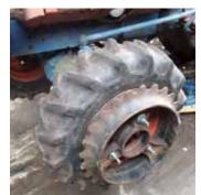
David Simpler's Kubota tractor was light on the front end, so he mounted two 16-in. cast iron Brillion cultipacker wheels dia. at 25 lbs. apiece on the front rims.
