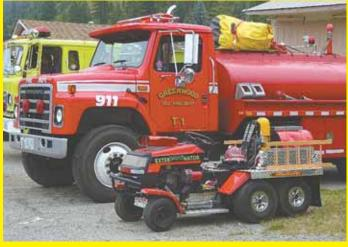
I built a mini firetruck for a local parade. It started life as a Craftsman 16 hp. mower. I replaced the blown Briggs & Stratton motor with a 621cc Kohler, and then added some hot rod parts - a blower hood scoop that works off the throttle, Harley Davidson short mufflers, and a deadman switch on a tether cord. I mounted an old fire department siren on it and "wig wag" LED lights. Friends made the hose beds and ladders. It
