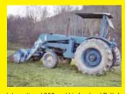
International 300 and big Leyland British tractor. Local welding shops refused the job because of liability so I hired a welder who used 1-in. thick stainless steel plates that bolt to the rear axle. The plates weld to 2 by 4 double-wall tubes. The steel top is framed with 2-in. sq. steel tubing.
