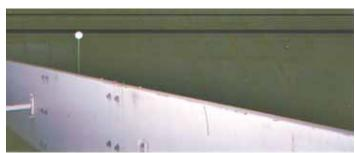
Golf ball mounts on a metal rod welded to top of wagon's gate opener. Rod goes up through lip at top of wagon. When golf ball is above lip, Fratzke knows gate is open.
