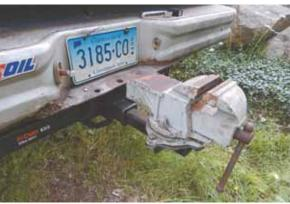
Bishop bolted a steel plate onto a vise and then welded the plate to a length of 2-in. sq. tubing, which fits into vehicle's receiver hitch.
