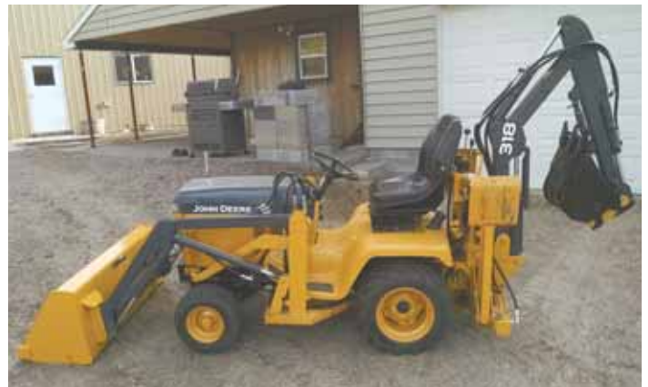
Jake Tolstedt's garden tractor loader and backhoe looks factory made, but he built it himself over a 3-year period.
