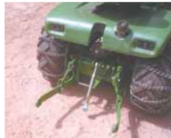
Kevin Ranette sells a 3-pt. hitch and front-mounted brush guard for Deere garden tractors. By removing a pin you can flip guard forward to access tractor's engine.
