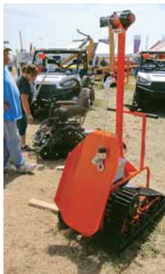
Action Trackporter is designed to remove dead hogs from confined areas. It rides on rubber tracks and comes with a stand-on platform on back.
