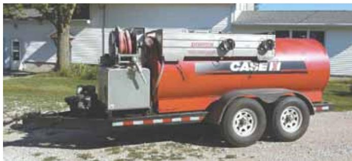
Home-built fuel trailer is equipped with a 1,000-gal. fuel tank, a 100-gal. tank for urea, and a tank for changing oil on an irrigation pump.
