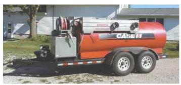
Home-built fuel trailer is equipped with a 1,000-gal. fuel tank, a 100-gal. tank for urea, and a tank for changing oil on an irrigation pump.
