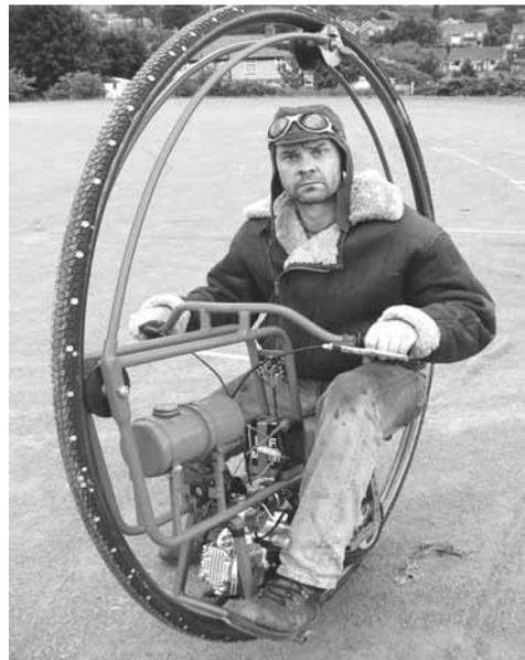
Dave Southall's home-built monowheel is basically 2 circles, one inside the other. The inner one uses an engine to drive the outer circle around it.
