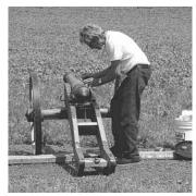
The 5-ft. long barrel was formed by building up layers of pipe, driving one inside the other for a tight fit.
