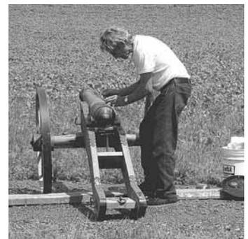
The 5-ft. long barrel was formed by building up layers of pipe, driving one inside the other for a tight fit.
