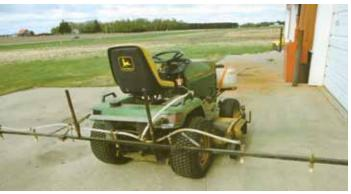
Lester Adelman's 3-section sprayer has a 14-gal. tank that mounts on front of his Deere 445 riding mower, and a 10-ft. breakaway boom on back.
