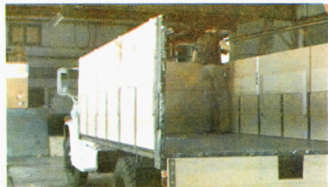
Specially designed box has hinged sides which drop for side loading or unloading of bagged seed and other materials. Converts from complete flatbed to grainbox in matter of minutes.
