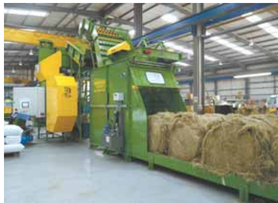
An English equipment manufacturer makes this baler/packer that mechanically repackages materials from big square or round bales.
