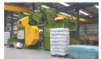
Machine tears the bale apart and then conveys the material into a baler, which packs hay into 40 to 60-lb. sealed plastic bags.
