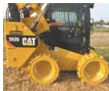
**Metal Skid Steer Wheels** - Inventor Derek Hird introduced metal wheels with staggered 2 by 9-in. cleats. The wheels have standard 6-in. inner hubs with 8 bolts so they just bolt on in place on skid steers fitted with 12 by 16.5-in. tires. ([www.evolution-wheel.com](http://www.evolution-wheel.com); ph 888 249-4790)
