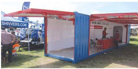
At a recent farm show, Schweiss Bi-Fold Doors showed how the side and end of a standard shipping container can be equipped with large one-piece, hydraulic-opened doors. "It opens up the entire container, making it much easier to access contents," says Mike Schweiss.
