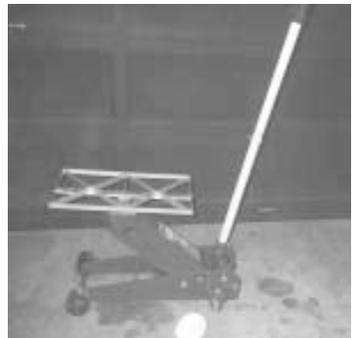
standard floor jack. It consists of a flat metal rack made from short pieces of strap iron. A metal shaft fits down into the jack. It slips on and off as needed. Quick and simple."
