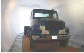
Giant containment bag completely encloses the work space, allowing workers to sandblast trucks, tractors and pickups, without making a mess. Bags hold their shape with low-pressure positive airflow from a blower.
