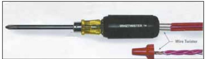
Wires are inserted into handle of screwdriver and then twisted together for a tight connection.
